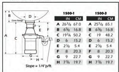
Sink Mounted Models with #2539 Sink Mount Installation
